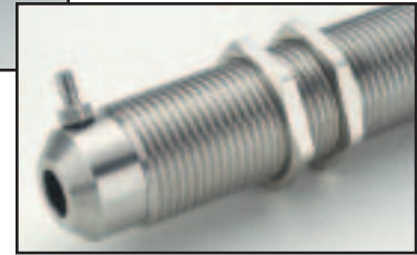
BELOW: M10L1V with standard air purge attachment in place, providing constant lens cleaning
